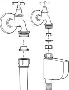
• Remove the nuts of the water intake hoses to clean the surfaces of the filters on the water intake valves with an appropriate brush.
